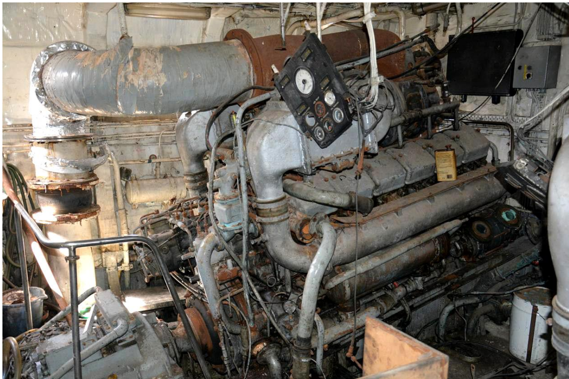
Right : Curl Curl's original MTU 493 TY71 super-charged marine diesels (top). Replacement options being considered are MTU 12V 2000 M72 (centre) and CAT C32 Acert (bottom) / ANDREW HEIGHWAY photo, all
