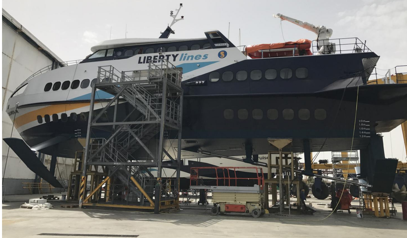
The third 32m Admiral 250 hydrofoil completed, Carmen M , at the Trapani shipyard earlier this month / LIBERTY SHIPYARD photo
