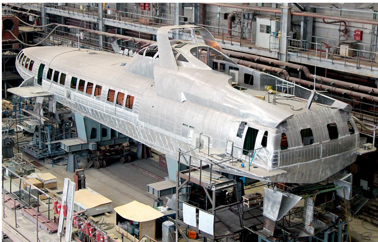
Top + Right: The prototype Kometa 120M under construction at the Vympel Shipyard at Rybinsk, Russia, late last year / VYMPPEL SHIPYARD photo, both
