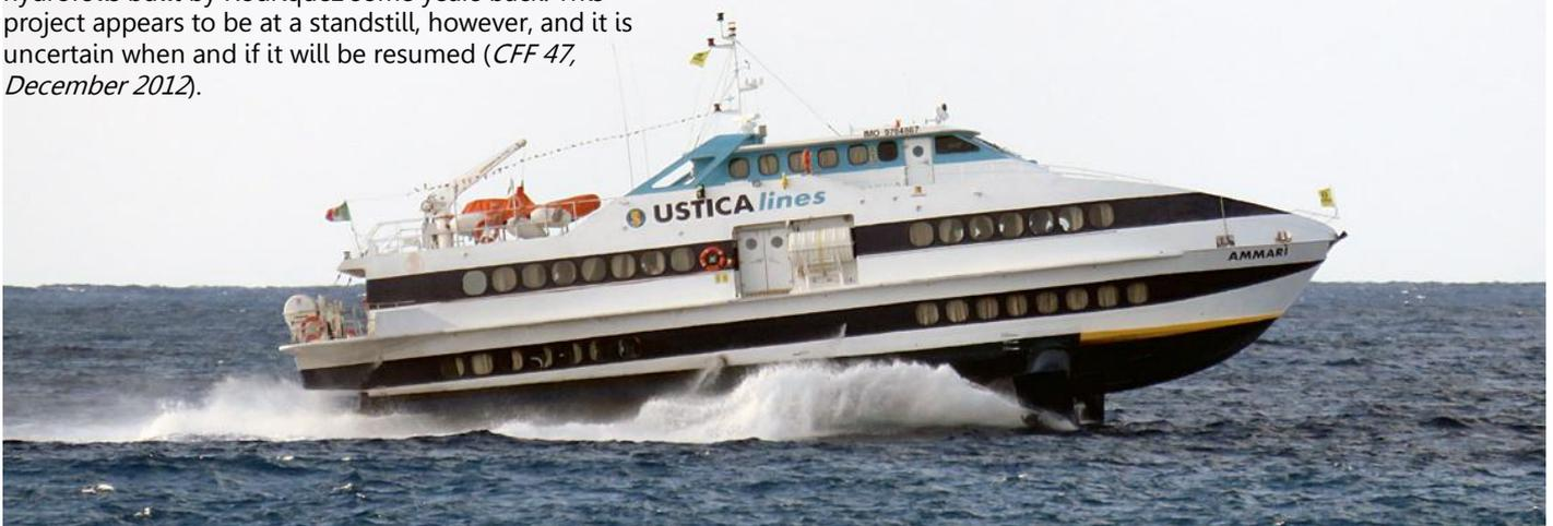
Power is supplied by a pair of 2,300kW engines positioned midships expected to offer a cruising speed of 37 knots and maximum speed of 38 knots. The range is 600 nautical miles.
